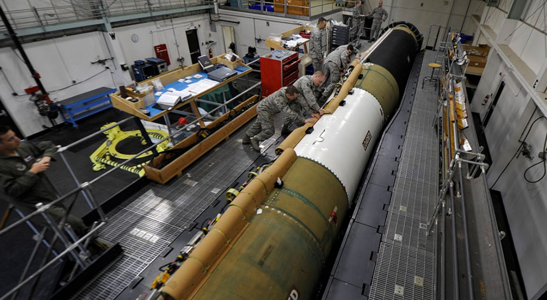
An aging Minuteman III missile, slated to be replaced by the new Ground-Based Strategic Deterrent system, is fitted with a new cable by members of the U.S. Air Force. (Photo by U.S. Air Force)
