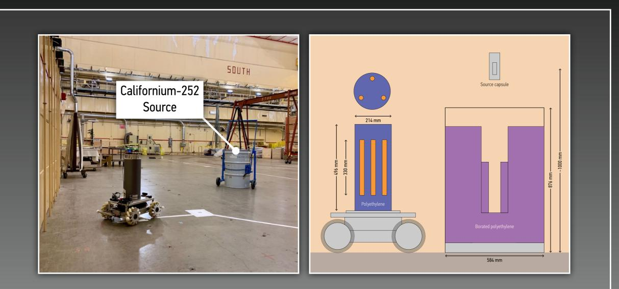
Boron-coated straw (BCS) detectors embedded in a polyethylene cylinder One 3-detector (pictured) and two 6-detector systems available Method for "single-shot" directional measurements Experimentally-benchmarked MCNP model
