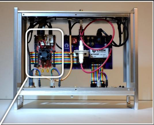
Red Pitaya single-board computer (<u>redpitaya.com</u>) Xilinx Zynq 7010, SoC with FPGA and ARM A9 14-bit ADC, 125 million samples per second
