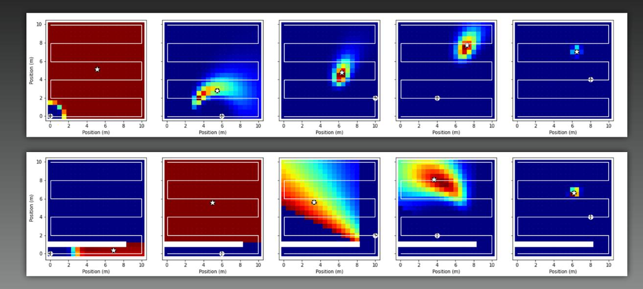
Robot follows a predefined raster pattern and updates particle weights with each measurement
