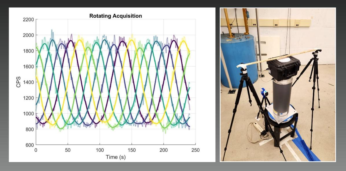
Measurements at Princeton Plasma Physics Laboratory, October 2022 using a PuBe source at PPPL's Calibration and Service Laboratory (CASL)
