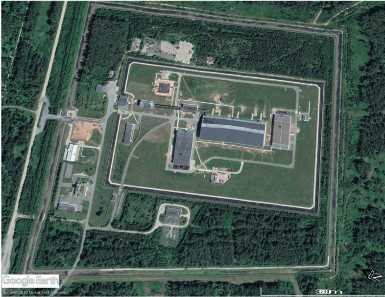
Figure 4. US-built USD 400-million storage facility for about 24 tons of excess Russian weapons plutonium outside Ozersk. Note the outer and inner security perimeters, which each have two fences with a microwave-beam monitored strip between. The storage building in the center is designed to withstand bombs and the cans of plutonium are stored in vertical tubes in a concrete monolith (Google Earth, 16 July 2019, 55.713° N, 60.848° E).
