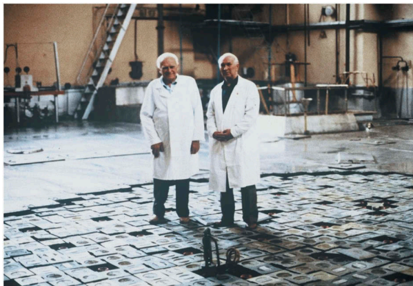
Figure 2. The managers of the “A” reactor stand on its top where cylindrical slugs of aluminum-clad natural uranium metal were loaded into vertical channels. After irradiation, the fuel was dropped out of the bottom of the tubes into a cooling pool before being reprocessed to recover the plutonium (NRDC).
