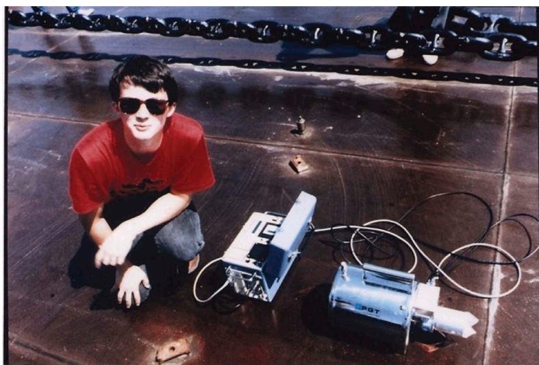
Figure 6. Steve Fetter, the technical lead on the FAS-NRDC team, with the NRDC gamma detector, a crystal of germanium that was kept cool with liquid nitrogen and attached by cable to a multichannel analyzer that plotted the spectrum of the energies deposited in the crystal (NRDC).
