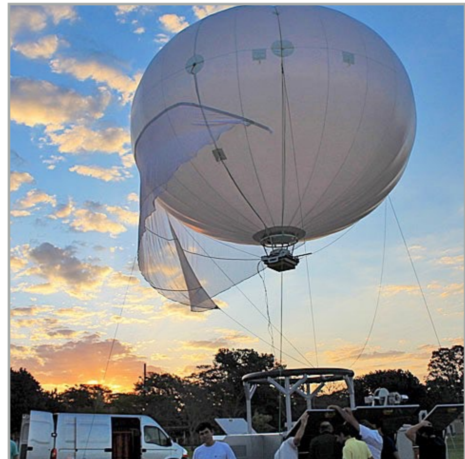
Tethered balloons for 24/7 site surveillance Widely used for civilian and military applications Credit: Altave Omni, www.altave.com.br
