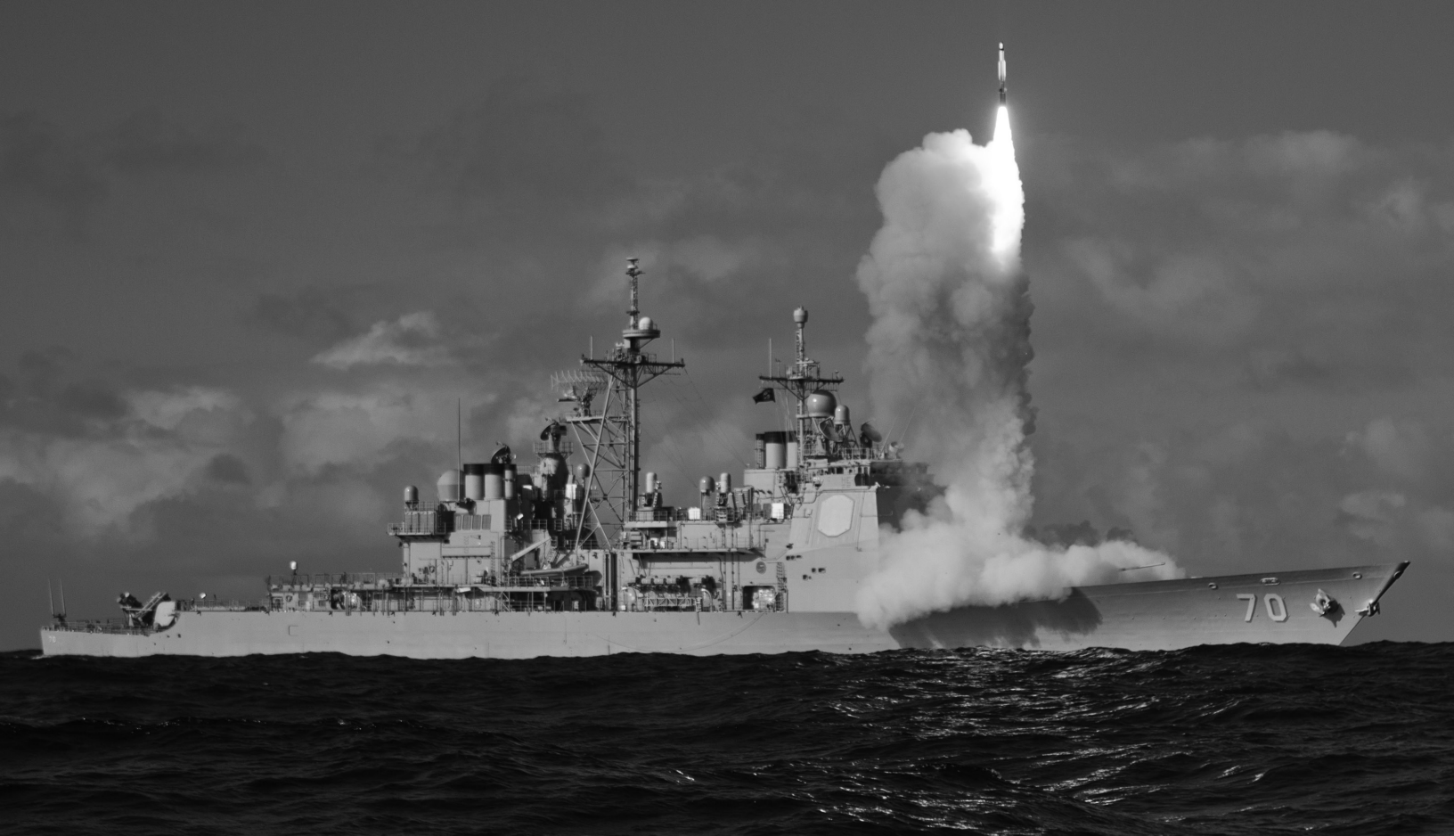
A Standard Missile-3 (SM-3) Block 1B interceptor is launched from the USS Lake Erie during a test in the mid-Pacific on May 16, 2013. The SM-3 Block 1B intercepted the target missile launched from the Pacific Missile Range Facility at Kauai, Hawaii. The ship, equipped with the second-generation Aegis BMD weapon system, detected and tracked the target using the onboard SPY-1 radar, visible to the left of the base of the plume. (Photo: Missile Defense Agency)
