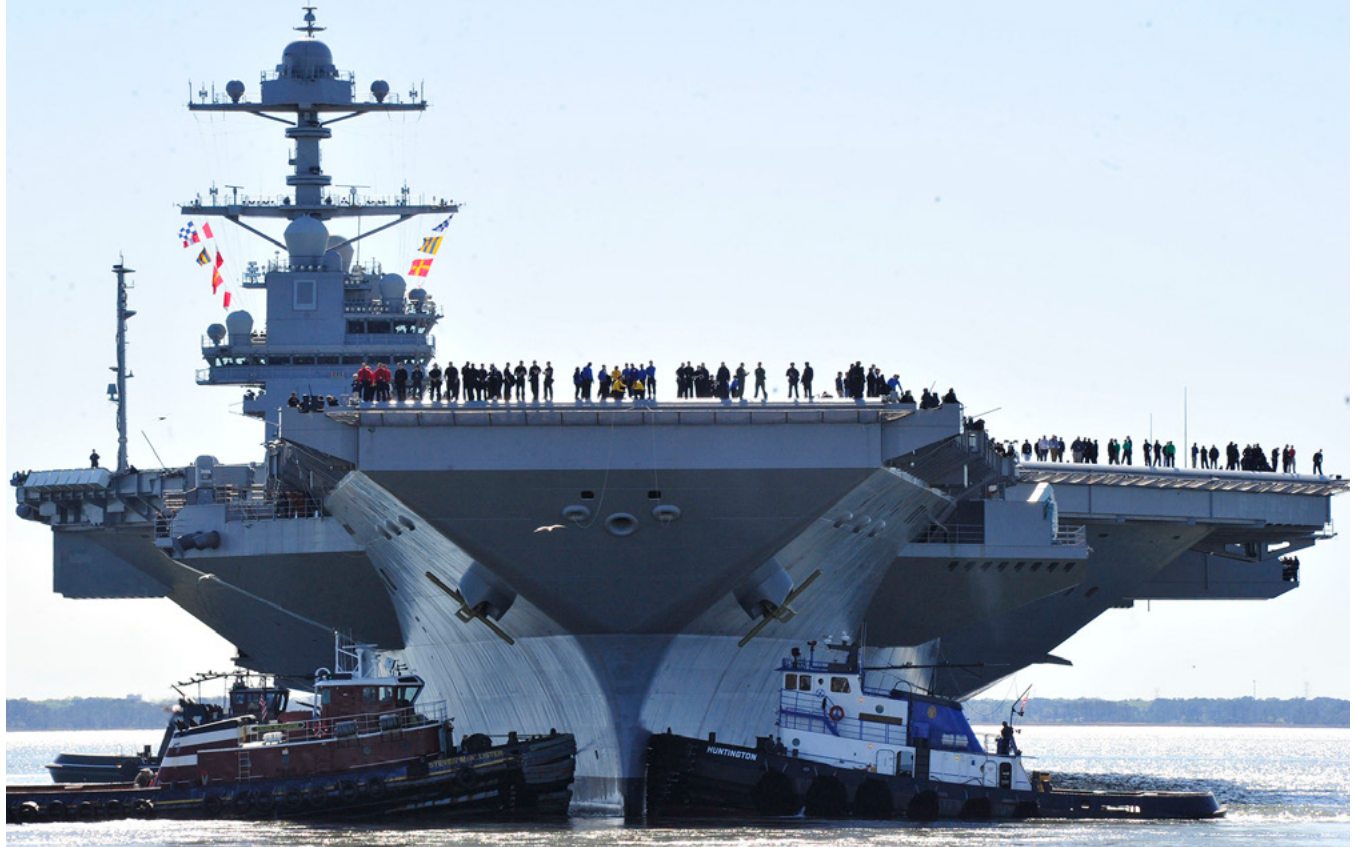
The USS Gerald R. Ford , the mostly recently commissioned U.S. aircraft carrier, is powered by two nuclear reactors fueled with weapon-grade uranium. Some other nations use low-enriched uranium to fuel their nuclear-powered naval vessels, and the U.S. Navy has assessed that it could also use low-enriched uranium for its aircraft carriers. (Photo: Christopher Delano/U.S. Navy via Getty Images)
